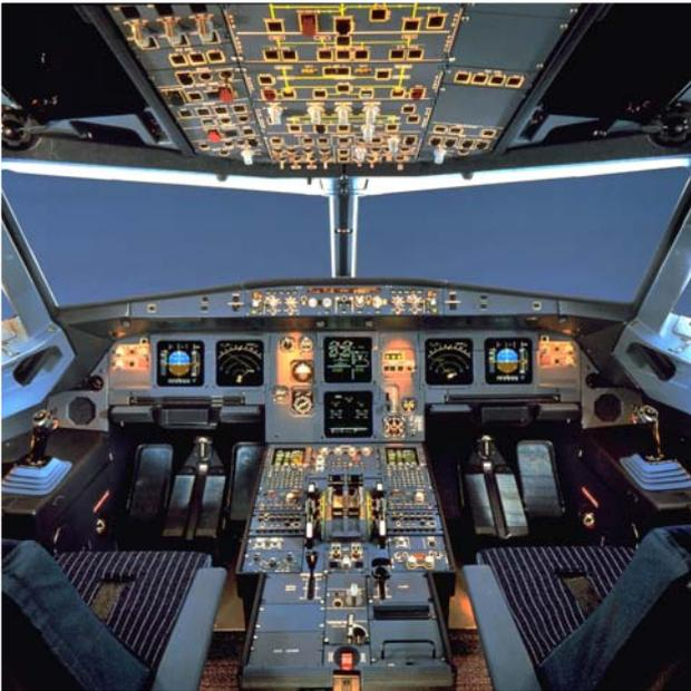
Figure 13: Glass cockpit and side stick control (Airbus A320)
