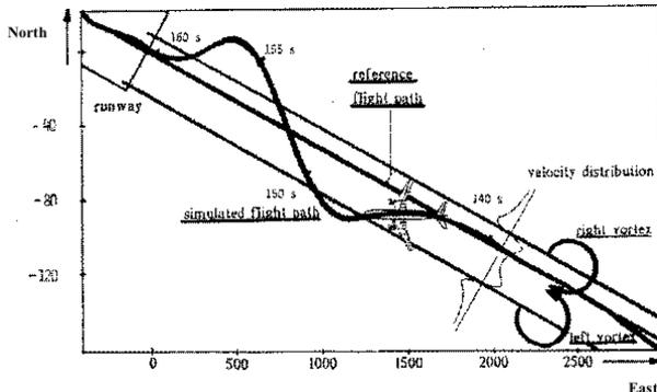
Figure 57: Simulated wake vortex encounter during final approach
