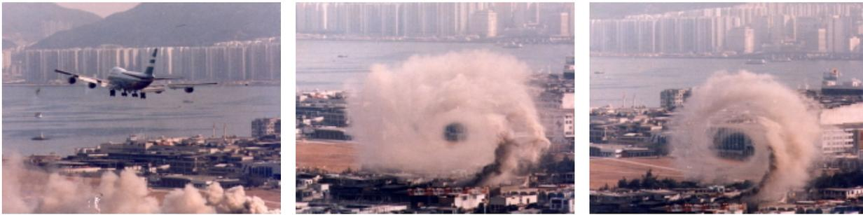
Figure 59: Rollup and decay of a wake vortex
