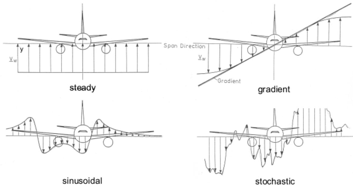
Figure 42: Local airspeed distribution when passing different basic wind and turbulence fields
