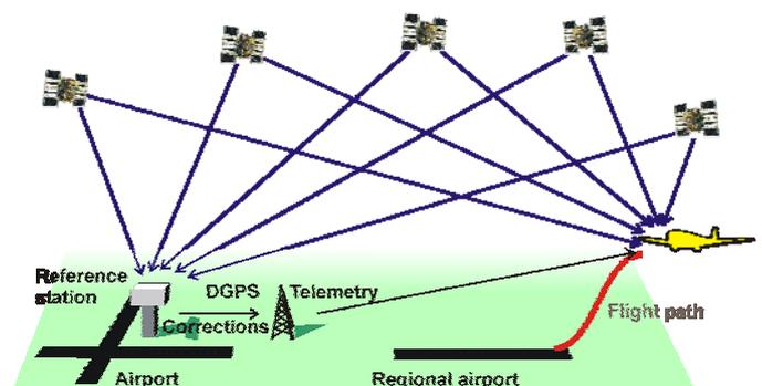
Figure 19: Differential satellite navigation principle
