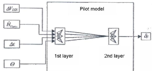
Figure 54: Artificial neural network architecture for a thrust control system.
