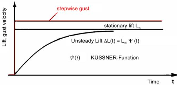
Figure 44: Unsteady lift response as a function of a stepwise gust (Küssner 1926)
