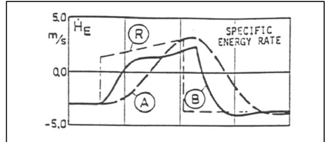
Figure 50: Required thrust (especially specific energy rate) in the wind shear of fig.49. - R required specific energy rate, A conventional automatic flight controls (low throttle activity, B specific energy rate management
