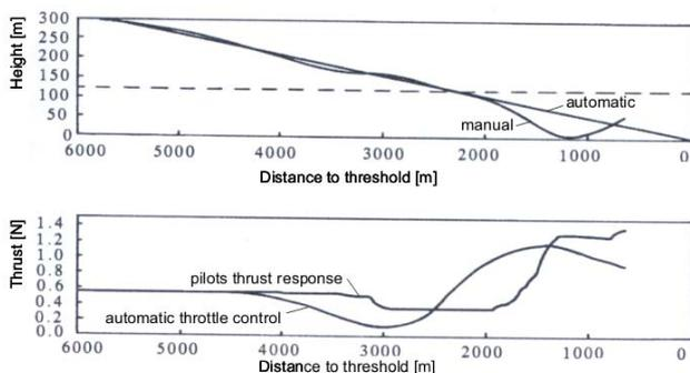
Figure 53: Simulated flight path and thrust response for the fatal Khabarovsk wind shear
