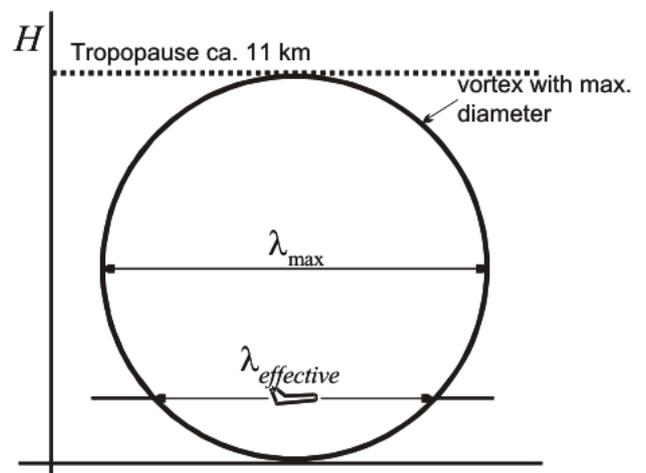
Figure 46: Effective and maximum turbulence wavelength.
