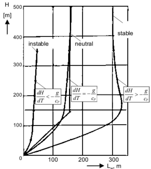
Figure 43: Integral scale  $L_w$  as a function of height and stability of the atmosphere
