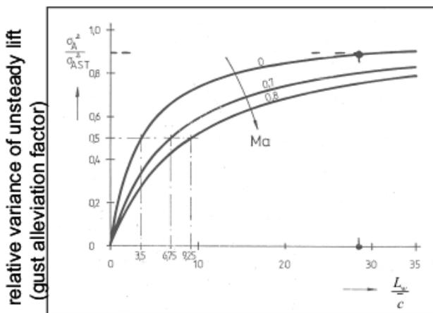
Figure 47: Gust alleviation factor as a function of relative integral scale  $L_w/c$ .
