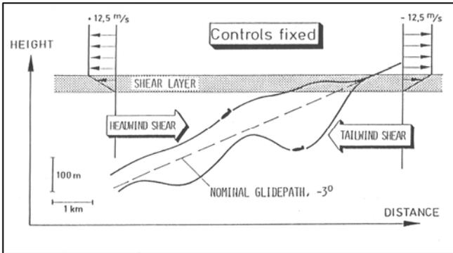
Figure 49: Typical aircraft response in a wind shear layer
